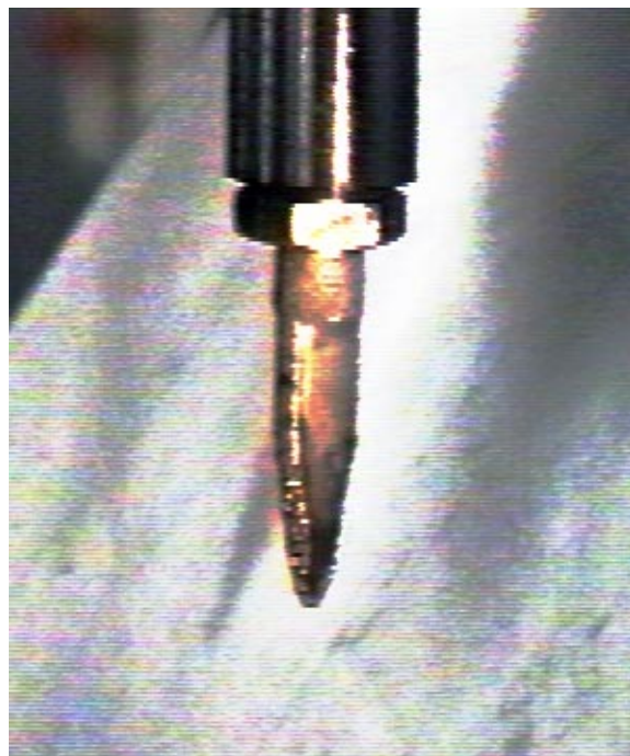
Figure 3. Drill Mounted in Collet
