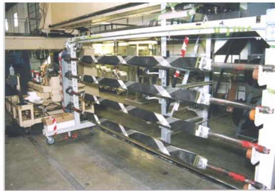
Figure 2: Filament Winding Dry Tow
