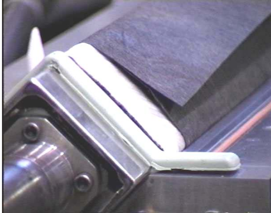
Figure 8: RTM Mold End Seal & Preform
